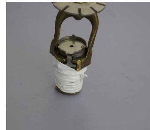
Sealing assembly blocking
