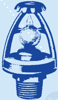
Grinnell system replaces the fusible link.
